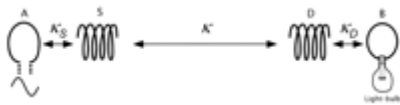
Fig. 1. Schematic of the experimental setup. A is a single copper loop of radius 25 cm that is part of the driving circuit, which outputs a sine wave with frequency 9.9 MHz. S and D are respectively the source and device coils referred to in the text. B is a loop of wire attached to the load (light bulb). The various \kappa s represent direct couplings between the objects indicated by the arrows. The angle between coil D and the loop A is adjusted to ensure that their direct coupling is zero. Coils S and D are aligned coaxially. The direct couplings between B and A and between B and S are negligible. [View Larger Version of this Image (8K GIF file)]
